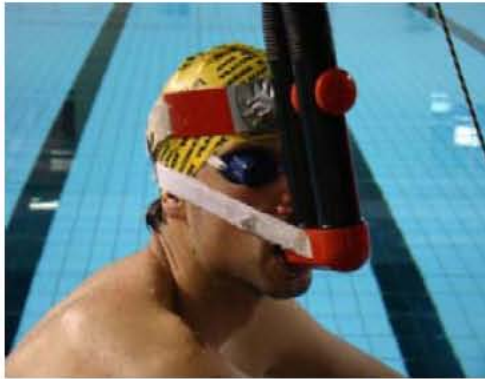
Fig. 1: Specific snorkel and valve system for breath-by-breath VO 2 kinetics assessment in swimming.
