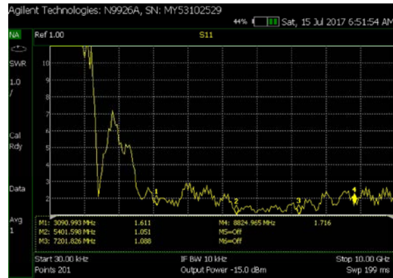
Fig. 18: Voltage standing wave ratio plot
