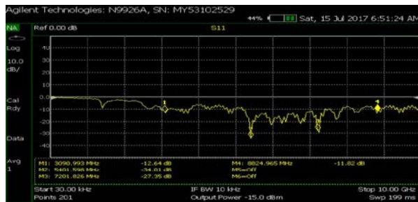
Fig. 17: Measurement return loss plot of proposed wideband antenna design
