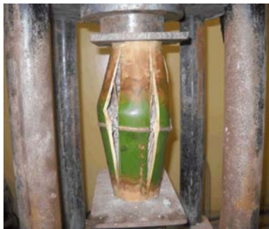
Fig. 3.4: (a) Reinforced Fresh Bamboo Under Compressive Test
