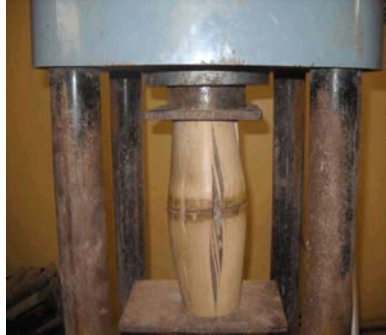
Fig. 3.4: (b) Reinforced Dried Bamboo Under Compressive Test
