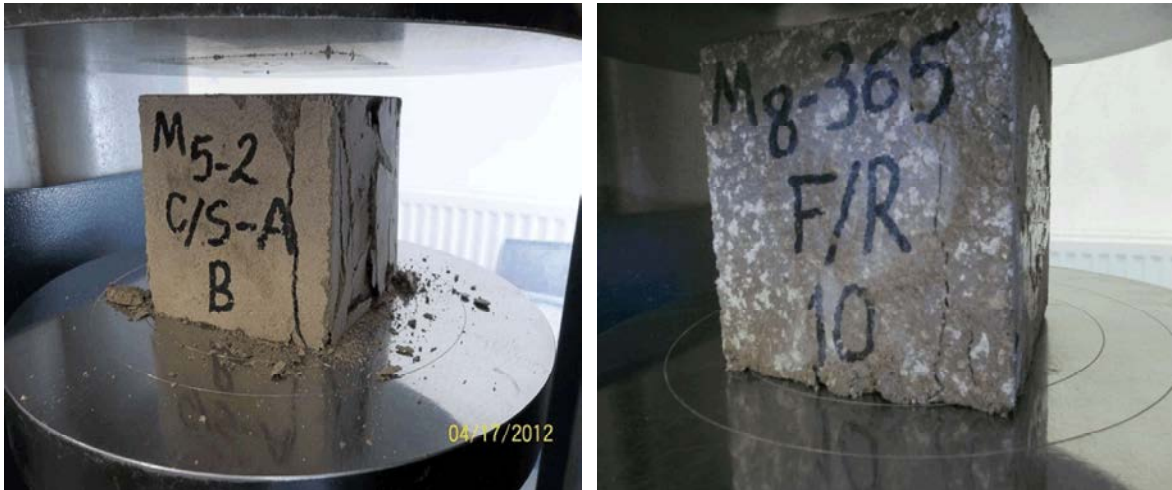
Fig. 7: Failure mode of control (left) and 100% SPS (right) concretes
