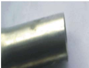
Fig. 1: As-cast Al-Mn alloy
