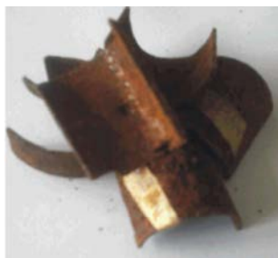
Fig. 2: Corroded pieces of Al-Mn alloy cut and exposed to sea water environment
