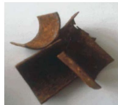
Fig. 2: Corroded pieces of galvanized steel cut and exposed to sea water environment
