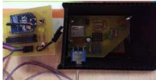
Fig. 7: Recharging circuit connected to the transponder circuit
