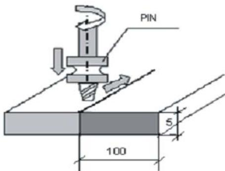
Fig. 1: Schematic diagram of FSW model
