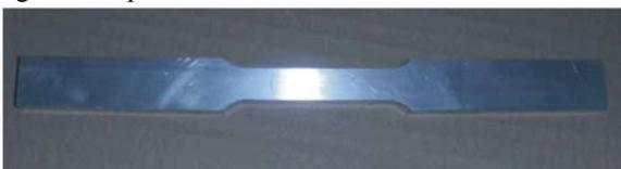
Fig. 5: Samples welded at 900 rpm
