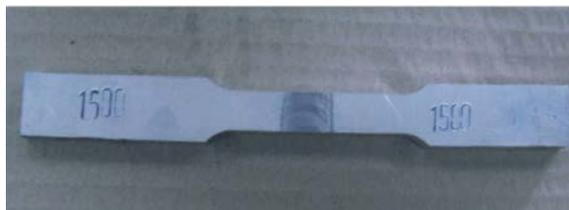
Fig. 7: Samples welded at 1500 rpm
