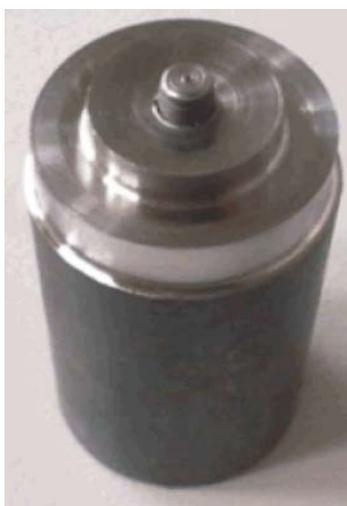
Fig. 2: Mixer pin used in FSW
