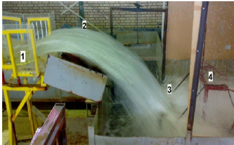
Fig. 2: Experimental setup, (1) Flip bucket, (2) peak of the jump, (3) jet impact location, (4) Platform
