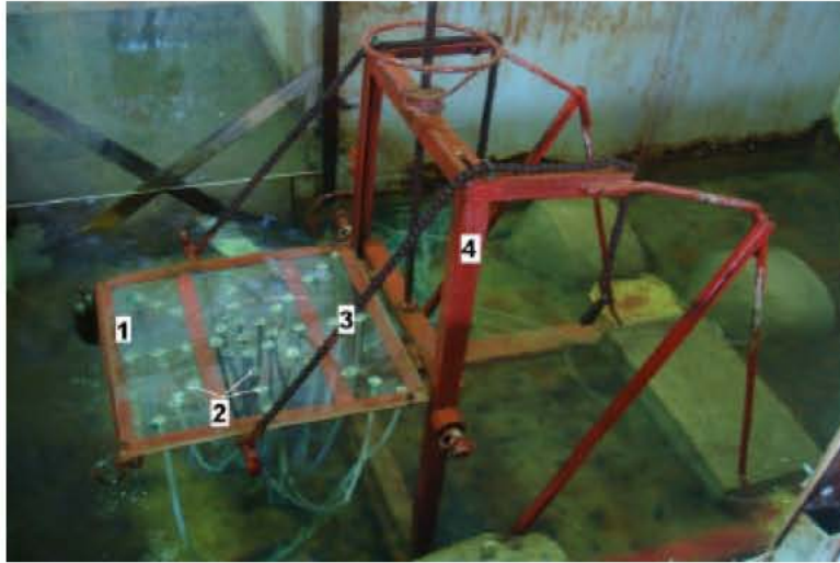
Fig. 3: (1) Flat plate, (2) Hollow, (3) Rotor arm, (4) platform
