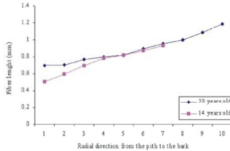
Fig. 5: The effect of age and radial position on the fiber length
