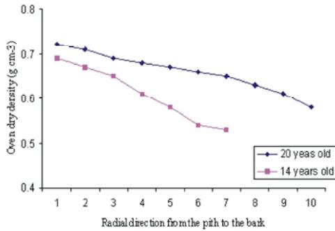
Fig. 1: The effect of age and radial position on oven dry density
