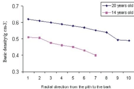
Fig. 2: The effect of age and radial position on the basic density
