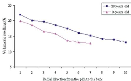
Fig. 4: The effect of age and radial position on the volumetric swelling
