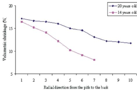
Fig. 3: The effect of age and radial position on the volumetric shrinkage
