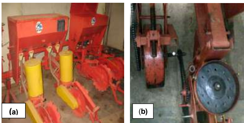
Fig. 1:(a) Test Planter (Model ATESPAR, GIAD Company) and (b) Seed metering mechanism
