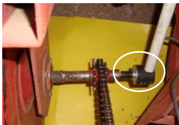
Fig. 5: Rotary Encoder Connection.
