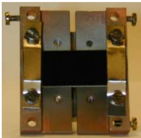
Fig. 3: Sample holder built with Ta and used for cleaning silicon sample inside the ultra high vacuum chamber.
