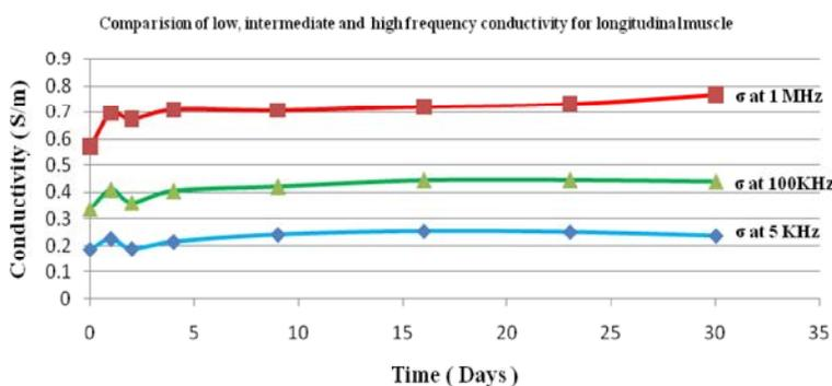
Fig. 8: (b) Conductivity (S m<sup>-1</sup>) of longitudinal muscle as a function of time post-irradiation (days). The curves at low (5 KHz), intermediate (100 KHz) and high frequency (1 MHz)
