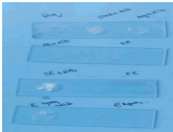
Fig. 7: Microscopic Slide method for understanding K.galanga extract interaction with albumin
