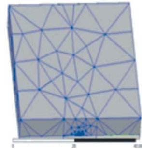
Fig. 2: Overall mesh of the antenna
