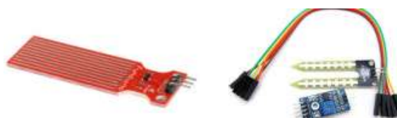
Fig. 5: Continuous Water level Sensor and moisture sensor
