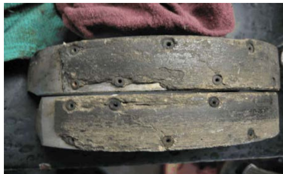
Fig. 1: Worn brake shoe
