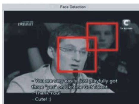
Fig. 3: Faces are being detected in the frame by using viola-jones algorithm. The red color square indicates the faces that are being detected
