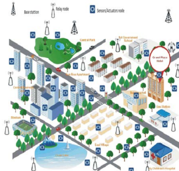
Fig. 2: Example of an unified deployment of sensor/actuator nodes, relay nodes and base station in an city environment.
