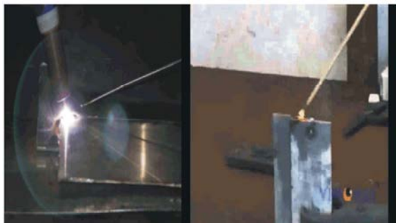
Fig: Welding of SS Plate
