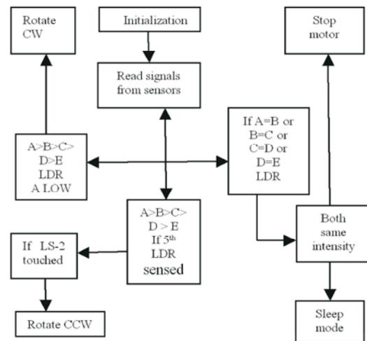
Fig. 2: Algorithm for PLC programming
