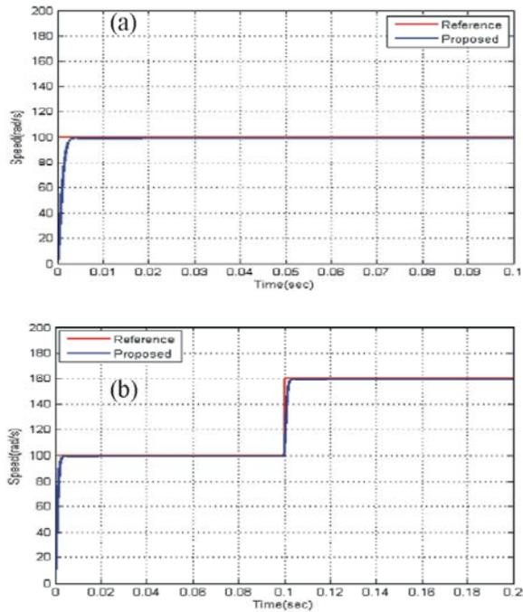
Fig. 5: Performance of the proposed MWNN-PSO based MRPID controller
