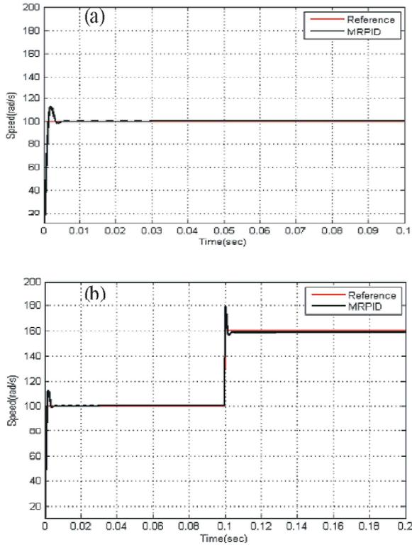
Fig. 4: Performance analysis of speed for the wavelet based MRPID controller
