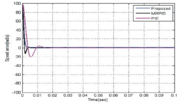
Fig. 7: Comparison of Error performance of various controllers
