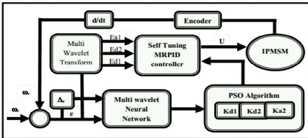
Fig. 1: Proposed Multi-wavelet neural network based MRPID controller
