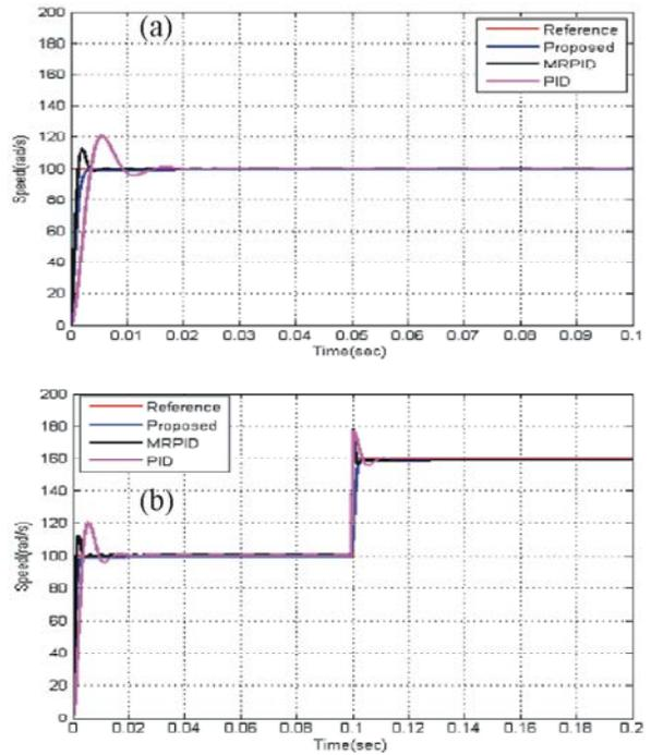
Fig. 6(a-b): Comparison analysis of the IPMSM drive controllers for step change and for the speed of 100 rad/sec
