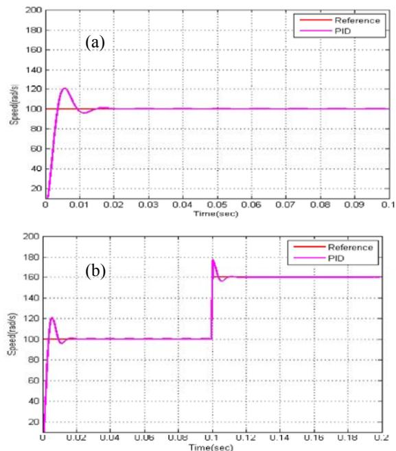
Fig. 3: Speed response of the IPMSM drive system using PID controller
