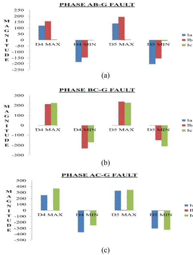
Fig. 8: Maximum and minimum detail coefficient of level 4 and level 5 in case of (a) AB-G, (b) BC-G, (c) AC-G
