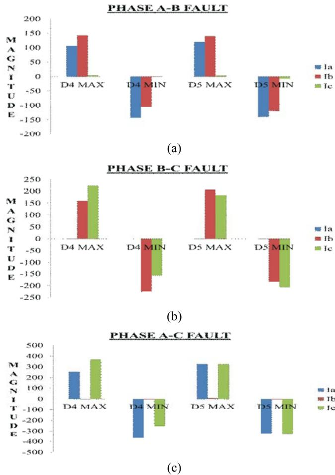
Fig. 7 Maximum and minimum detail coefficient of level 4 and level 5 in case of (a) A-B, (b) B-C, (c) A-C fault condition.
