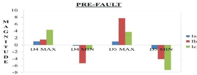
Fig. 5: Maximum and minimum detail coefficient of level 4 and level 5 in case of pre-fault condition
