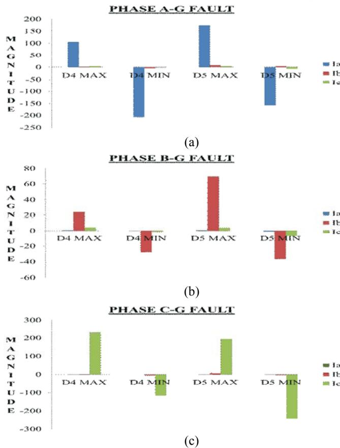
Fig. 6 Maximum and minimum detail coefficient of level 4 and level 5 in case of (a) A-G, (b) B-G, (c) C-G fault condition
