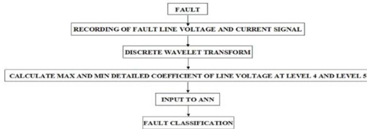
Fig. 1: Flow chart of the proposed approach for fault detection and classification
