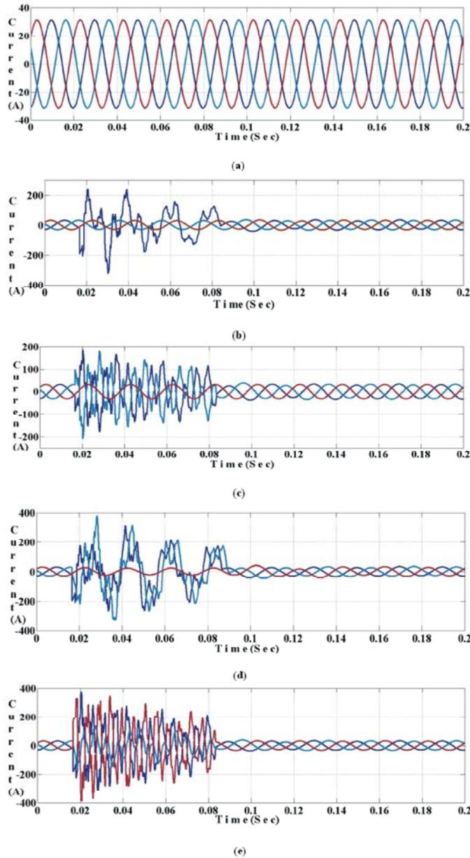
Fig. 4: Simulated Result for (a) Normal Condition, (b) Phase A to Ground, (c) Phase A to B, (d) Phase AB to Ground, (e) Phase ABC
