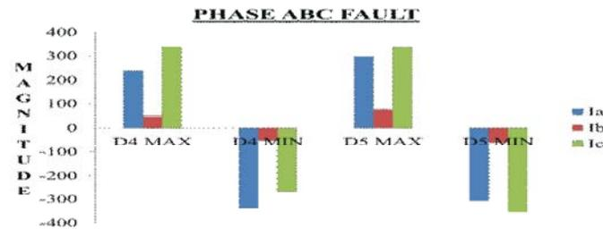
Fig. 9: Maximum and minimum detail coefficient of level 4 and level 5 in case of ABC fault condition
