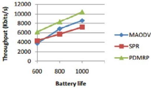
Fig. 5: Throughput versus battery life
