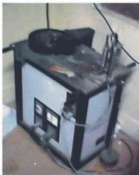
Fig. 5: Pin on disc machine
