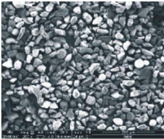
Fig. 11: SEM image of Al<sub>2</sub>O<sub>3</sub> at 200x magnification
