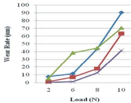
Fig. 14: Effect of Load on Wear rate
