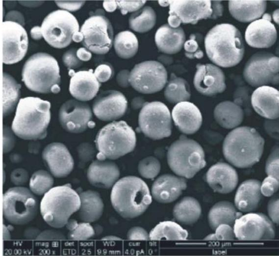
Fig. 10: SEM image of TiO<sub>2</sub> at 200x magnification
