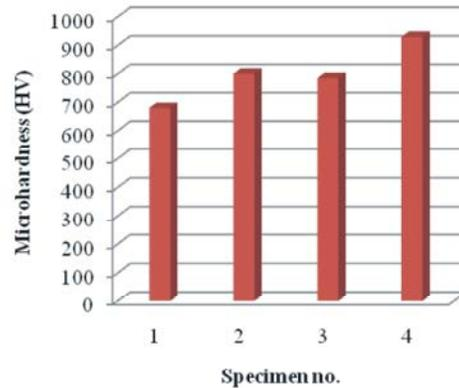
Fig. 13: Hardness values of coated specimens
