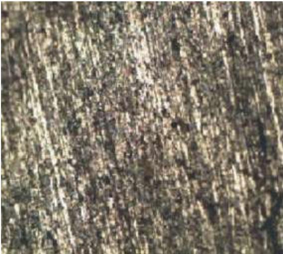
Fig. 4: Micro structure of AISI1040 Forged Steel – Before coating
