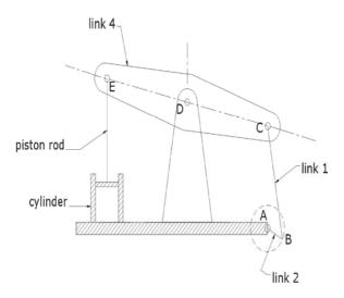
**Grashof Condition:** The grashof condition is used when analyzing KINEMATIC CHAINS for a four-bar linkage, the grashof condition is satisfied if  $S + L \le P+Q$  where S is the shortest link, L is the longest and P and Q are the other links [2]. When the grash of condition is satisfied, at least one link will be completely rotatable.
