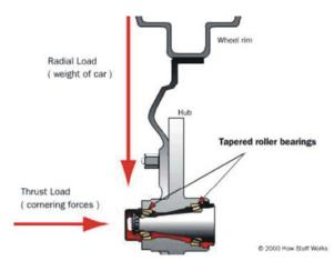
Tapered roller bearings are designed to support large radial and large thrust loads. These loads can take the form of constant loads or shock loads. Tapered roller bearings are used in many car hubs, where they are usually mounted in pairs facing opposite directions. This gives them the ability to take thrust loads in both directions. The cutaway taper roller on the left shows the specially designed tapered rollers and demonstrates their angular mounting which gives their dual load ability.
