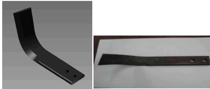
Fig. 5: Geometry (3D Model) the developed Blade
