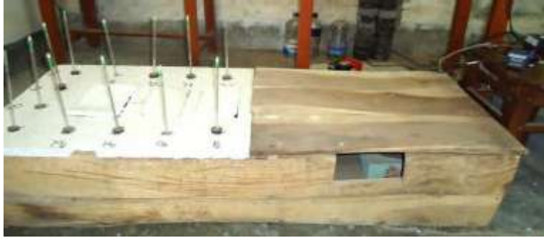
Fig. 1: Experimental setup of early age autogenous shrinkage at elevated temperature
