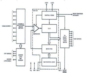
**Multiplexer:** The device contains an 8-channel singleended analog signal multiplexer. A particular input channel is selected by using the address decoder. Table 1 shows the input states for the address lines to select any channel [5]. The address is latched into the decoder on the low-to-high transition of the address latch enable signal.
