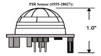
The PIR (Passive Infra-Red) Sensor is a pyroelectric device that detects motion by measuring changes in the infrared levels emitted by surrounding objects. This motion can be detected by checking for a high signal on a single I/O pin.
