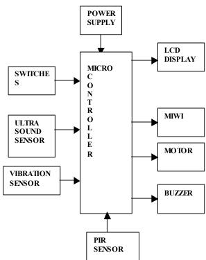
**Explanation:** In our project we have microcontroller, vibration sensor, PIR sensor, switches, power supply unit, MiWI, LCD and buzzer. Microcontoller is the entire controlling unit. The data's are transmitted and received through MiWi protocol.
