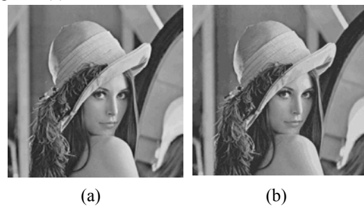
Fig. 2: Lena images of (a) original image with 256 gray level (b) clustered image with 12 gray-level
