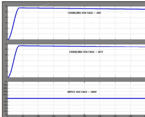
Fig. 11: Output and input voltage waveforms for reverse mode
