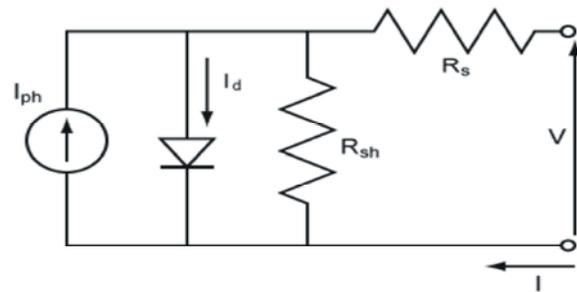
Fig. 3: Solar cell – Equivalent Circuit
