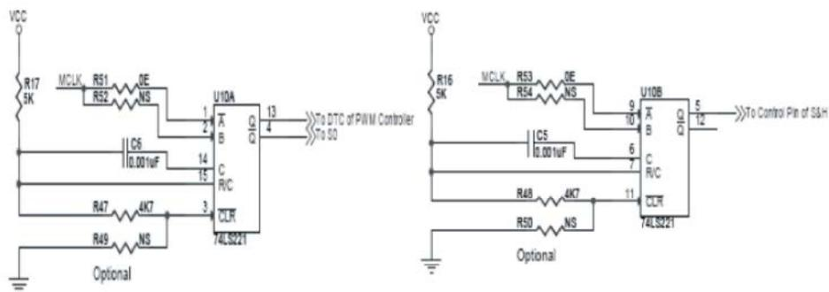
Fig. 8: Circuit diagram of trigger circuit
