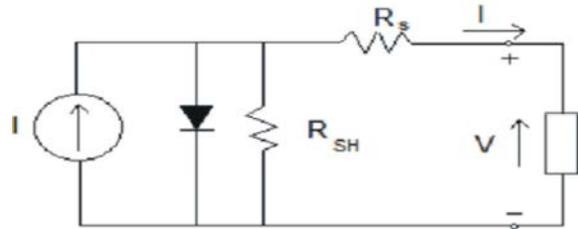
Fig. 1: Single diode model of a PV cell
