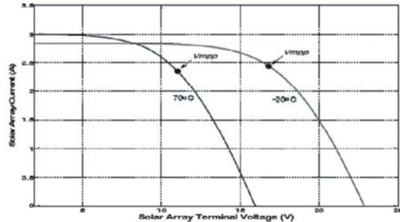
Fig. 2: I-V Characteristics of a solar panel
