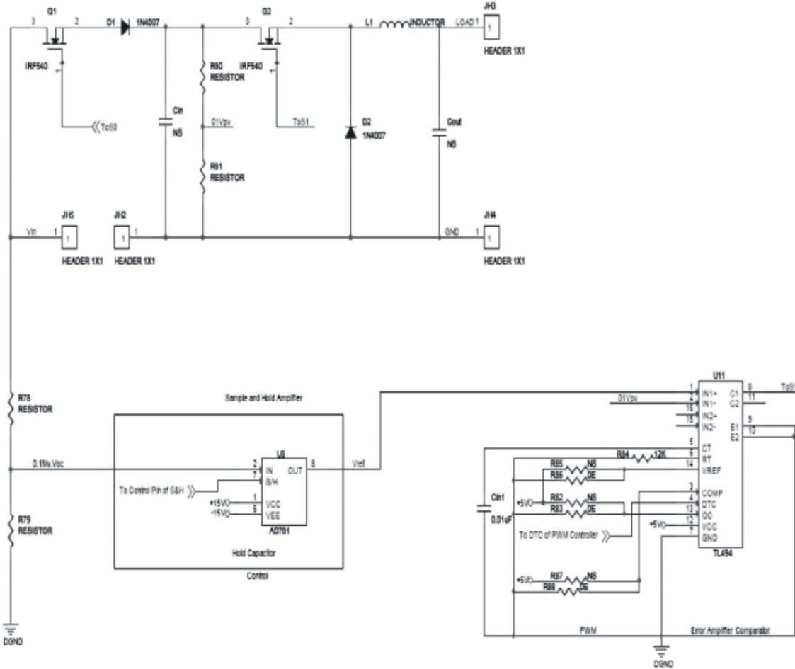
Fig. 9: Sample & Hold Amplifier in Harvester Platform
