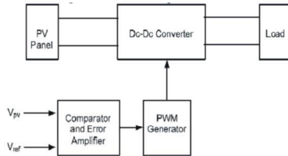
Fig. 4: Block Diagram of Voltage based MPPT
