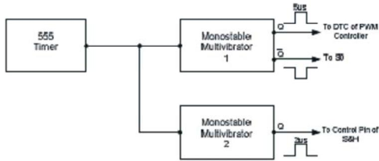
Fig. 7: Block diagram of the circuit controlling the sampling interval and the sampling period
