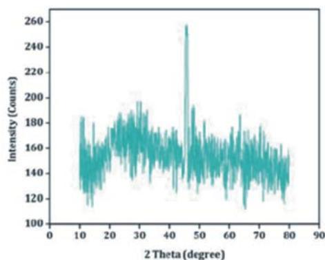
Fig. 3: XRD pattern of Iron Nanoparticles
