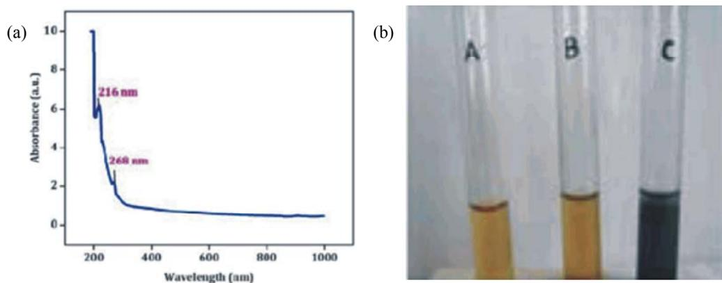
Fig. 2: a)- Iron Nanoparticle at 216-268 nm, b) Mixing of plant Bud extract with 0.001 M FeCl<sub>3</sub> Solution to get a reduced solution. Tube A- Ferric Chloride, Tube B- Clove Bud Extract, Tube C- Iron nanoparticle synthesized solution.
