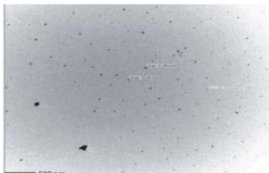
Fig. 11: TEM Image of METACHLOROANILINE/ c-MWCNTs
