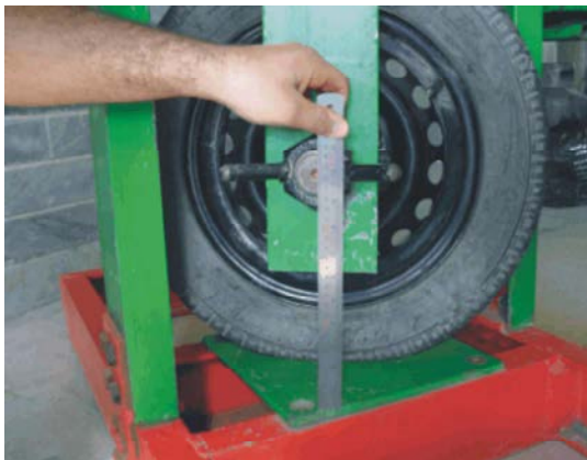
Fig. 3: Measuring static loaded radius
