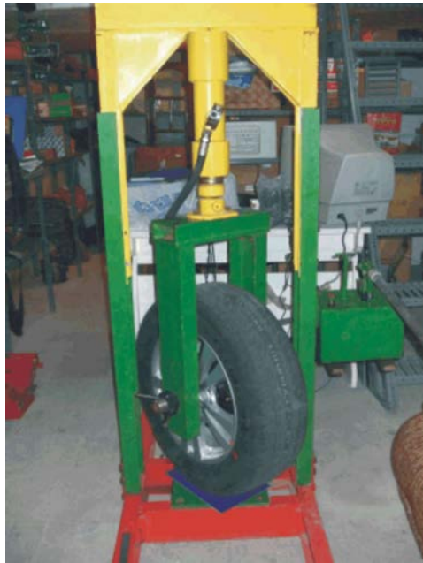
Fig. 2: Tire deflection test apparatus
