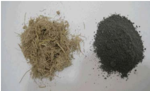
Fig. 3: Baggase on right and baggase ash products on left after grinding
