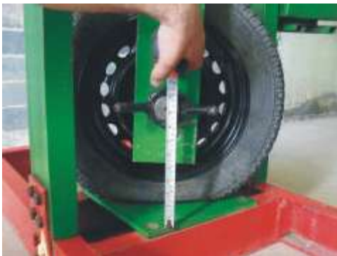
Fig. 3: Measuring static loaded radius
