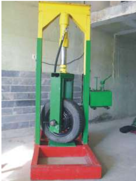
Fig. 2: Tire deflection test apparatus
