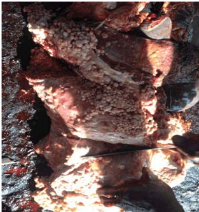
Fig. 4: Scrapping off tubercles
