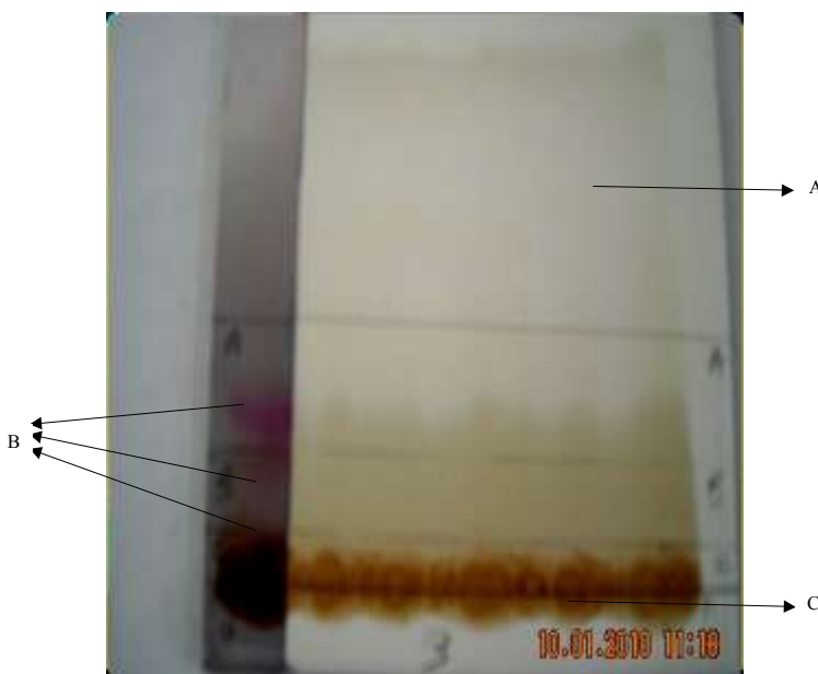
Plate I: Spotted TLC plate (A) with extract and developed in locating agent, B= bands of constituent located, C= spot base line
