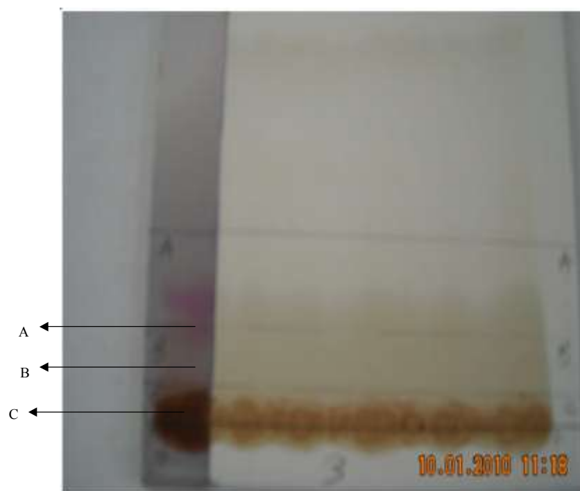
Plate II: TLC showing the location of the active constituents A, B and C scrapped
