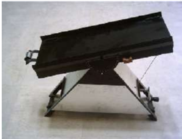
Fig. 3: Apparatus for measuring static coefficient of friction
