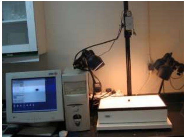
Fig. 2: Apparatus for measuring dimensional characteristics, area meter Delta-T England
