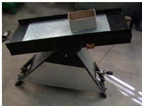
Fig. 1: Apparatus to determine coefficient of static friction
