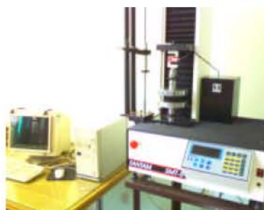
Fig. 3: Universal testing machine (Model santam SMT-5)
