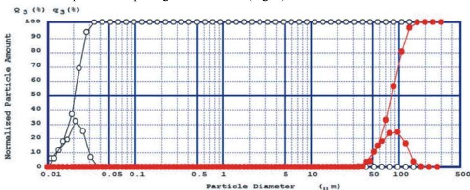
Fig. 1: Integral and differential particle size distributions of sulfur particles obtained: (o) - from calcium polysulfide, average particle size is 20 nm; • - after grinding in roller mill, average particle size is 70 micron.
