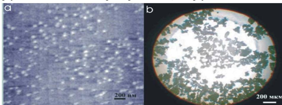
Fig. 2: Images of nanoparticles of sulfur (a) with an average size of 50 nm obtained with a scanning probe microscope and sulfur particles after grinding in roll mill (b) having an average size of 40 microns obtained by an optical microscope.
