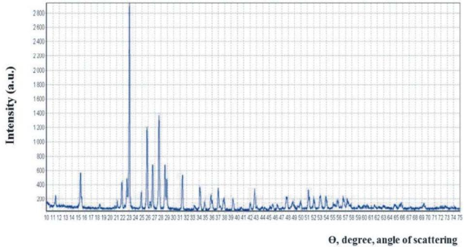
Fig. 3: XRD pattern of sulfur nanoparticles.
