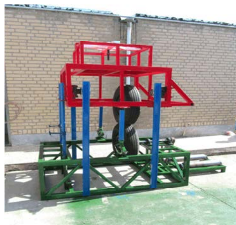
Fig. 3: Tire contact length measurement apparatus
