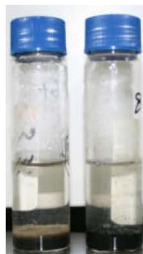
Fig. 2: Conversion of the activated sludge to black color under anaerobic due to formation of ferrous sulfide ( FeS ) and Pyrite ( FeS_2 ). Left tube: Control. The produced H_2S was pulled and measured using Dräger Mini Warn.
