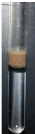
Fig. 3: Sludge rising test. At the end of the aerobic digestion, 10 ml was transferred to glass tube and left vertically for four hours at room temperature and observed visually. Raising of the of the biomass is an indication of anaerobic metabolism and production of N 2 and N 2 O as endproducts which causes decrease of the flocs density due to accumulation of the gases.
