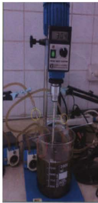
Fig. 1: The activated sludge bioreactor used in this study. The pH was maintained at about pH 7.5 using 0.25 M NaOH and 0.25 M HCl. The solution was mixed using suitable mixer and sterile oxygen was supplied using air pump to give oxygen content of 2 mg/l. The aerobic digestion was done at room temperature for 19 h.
