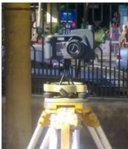
Fig. 5: Fixation of the GPS camera over the tripod
