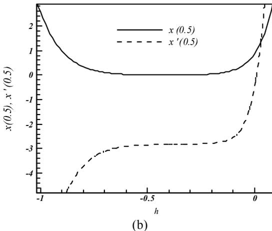
Fig. 1: The  $h$  curves to indicate the convergence region, (a)  $\alpha = 1, \beta = 1$ , (b)  $\alpha = 2, \beta = 2$
