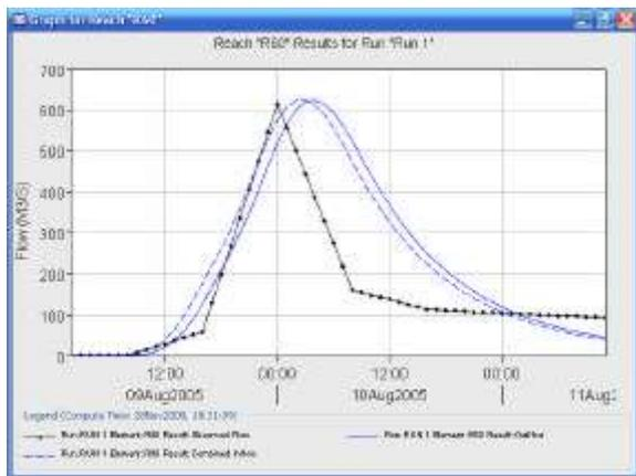
Fig. 7: Observed and calculated hydrograph in Tangrah station
