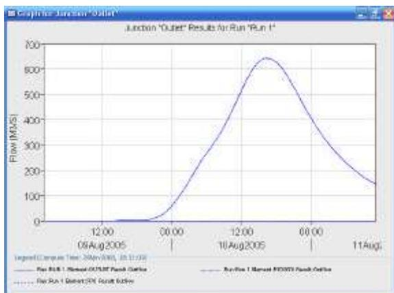
Fig. 8: Calculated hydrograph in outlet of basin
