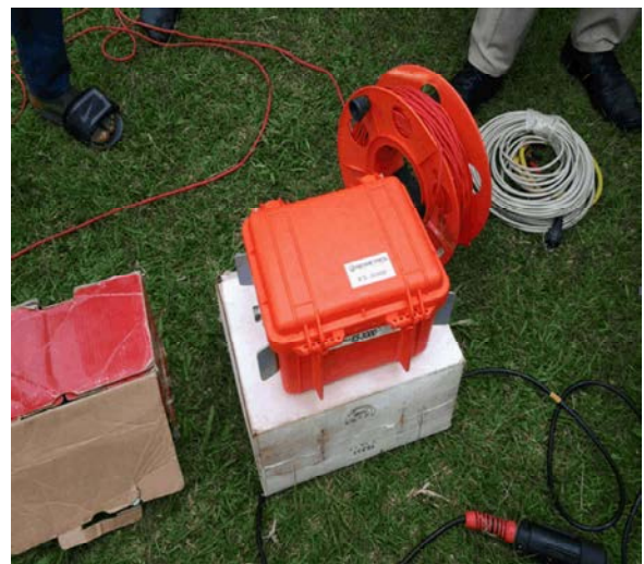
Plate 4: Geophone Cables connected to Seismogram
