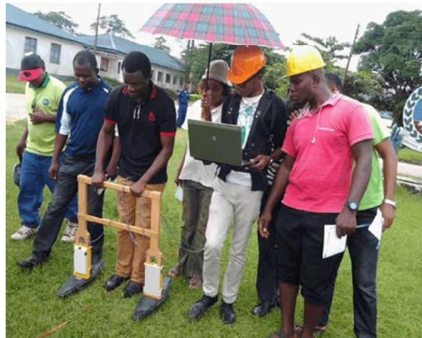
Plate 2: Transmitter and Receiver Antenna to the Radargram and Monitor (Field Lay Out)
